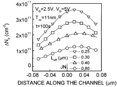
Fig. 2. Interface-state density ( $\Delta N_{it}$ ) profiles along the channel as a function of channel length. Stressing was done at  $V_G = 2.5$  V,  $V_D = 5$  V, for 100 s. The origin is chosen at the drain junction (JN), and the gate edge (GE) is at  $0.1 \mu\text{m}$ .
