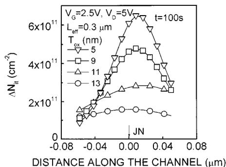
Fig. 4. Interface-state density ( $\Delta N_{it}$ ) profiles along the channel as a function of oxide thickness. Stressing was done at  $V_G = 2.5$  V,  $V_D = 5$  V, for 100 s. The origin is chosen at the drain junction (JN), and the gate edge is at 0.1  $\mu$ m.
