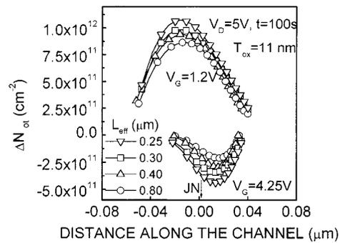
Fig. 3. Oxide trapped charge density ( $\Delta N_{ot}$ ) profiles along the channel as a function of channel length. Stressing was done at  $V_G = 1.2$  and 4.25 V,  $V_D = 5$  V, for 100 s. The origin is chosen at the drain junction (JN), and the gate edge is at  $0.1 \mu\text{m}$ . Electron trapping is shown in the negative scale.
