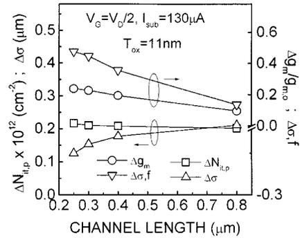
Fig. 8. Interface-state density peak ( $\Delta N_{it,p}$ ), spread ( $\Delta\sigma$ ) (left  $y$  axis), normalized peak transconductance degradation ( $\Delta g_m/g_{m,o}$ ), and fraction of the degraded channel ( $\Delta\sigma, f$ ) (right  $y$  axis) as a function of channel length ( $L_{eff}$ ). Stressing was done at  $V_G = V_D/2$ ,  $I_{sub} = 130$   $\mu\text{A}$  for 100 s on a transistor having  $T_{ox} = 11$  nm.
