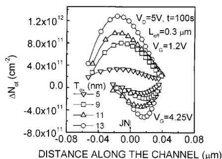
Fig. 5. Oxide trapped charge density ( $\Delta N_{ot}$ ) profiles along the channel as a function of oxide thickness. Stressing was done at  $V_G = 1.2$  and 4.25 V,  $V_D = 5$  V, for 100 s. The origin is chosen at the drain junction (JN), and the gate edge is at 0.1  $\mu$ m. Electron trapping is shown in the negative scale.
