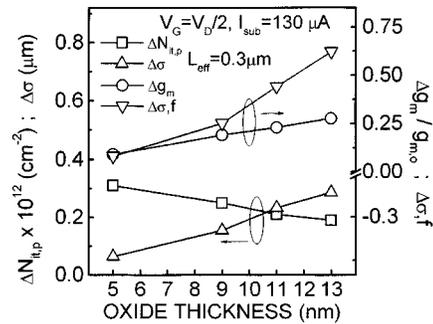
Fig. 9. Interface-state density peak ( $\Delta N_{it,p}$ ), spread ( $\Delta\sigma$ ) (left  $y$  axis), normalized peak transconductance degradation ( $\Delta g_m/g_{m,o}$ ), and fraction of the degraded channel ( $\Delta\sigma, f$ ) (right  $y$  axis) as a function of oxide thickness ( $T_{ox}$ ). Stressing was done at  $V_G = V_D/2$ ,  $I_{sub} = 130$   $\mu\text{A}$  for 100 s on a transistor having  $L_{eff} = 0.3$   $\mu\text{m}$ .
