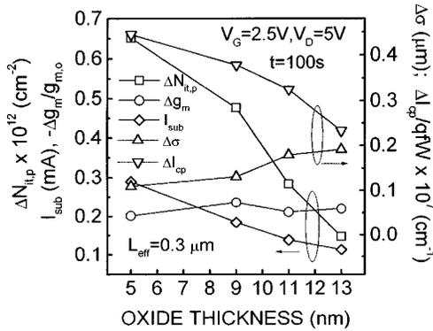
Fig. 7. Interface-state density peak ( $\Delta N_{it,p}$ ), substrate current during stress ( $I_{sub}$ ), normalized peak transconductance degradation ( $\Delta g_m/g_{m,o}$ ) (left  $y$  axis), interface-state density spread ( $\Delta\sigma$ ), and incremental charge pumping current ( $\Delta I_{cp}$ ) (right  $y$  axis) as a function of oxide thickness ( $T_{ox}$ ). Stressing was done at  $V_G = 2.5$  V,  $V_D = 5$  V for 100 s on a transistor having  $L_{eff} = 0.3$   $\mu\text{m}$ .
