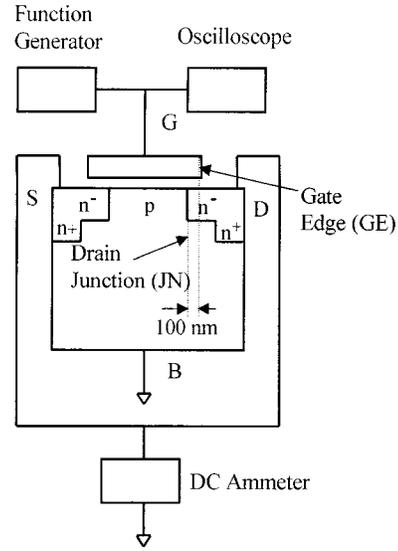
Fig. 1. Charge pumping setup along with the schematic diagram of the MOSFET used in the study showing drain junction (JN), gate-LDD overlap, and gate edge (GE).
