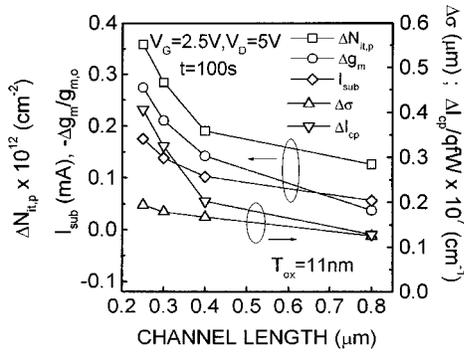
Fig. 6. Interface-state density peak ( $\Delta N_{it,p}$ ), substrate current during stress ( $I_{sub}$ ), normalized peak transconductance degradation ( $\Delta g_m/g_{m,o}$ ) (left  $y$  axis), interface-state density spread ( $\Delta\sigma$ ), and incremental charge pumping current ( $\Delta I_{cp}$ ) (right  $y$  axis) as a function of channel length ( $L_{eff}$ ). Stressing was done at  $V_G = 2.5$  V,  $V_D = 5$  V for 100 s on a transistor having  $T_{ox} = 11$  nm.
