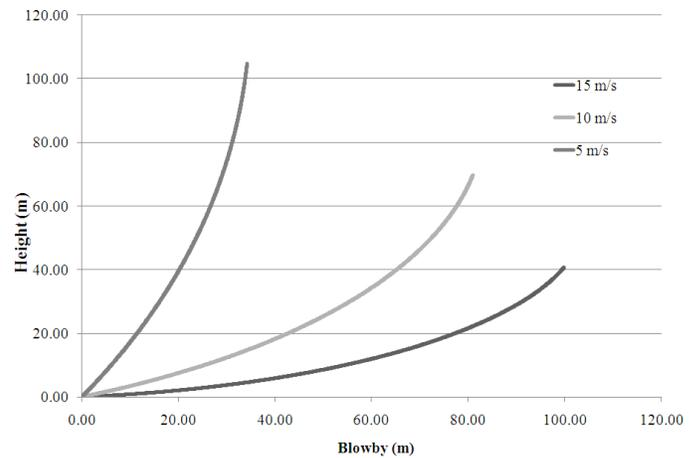
Figure 3. Tether profiles for various wind speeds from the mooring point
