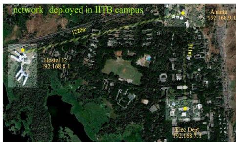
Figure 5. Wireless network setup in IIT Bombay campus
