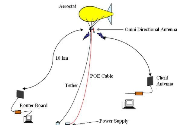
Figure 1. Conceptual Sketch of the overall system
