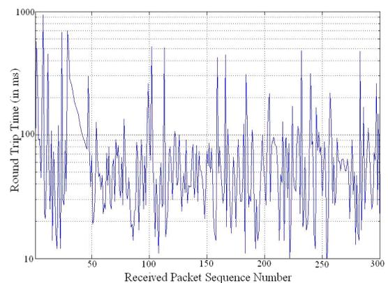
Figure 6. Round Trip Time as a function of Received Packet Sequence Number. The graph shows the ping statistics for packet numbers 0 to 300 sent over 7 Kms link between BS and Client.
