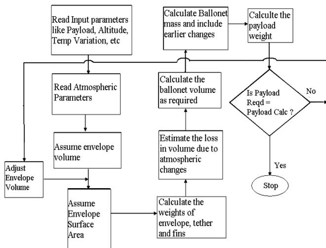
Figure 2. Flow Chart of the aerostat design methodology [5]
